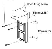
\*In case of indoor installation, the hood can be removed if it is not required.
