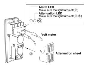
\*After adjustment, remove the attenuation sheet.
